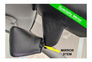
**STEP 5** - While sitting in the passenger seat, place the mount over the mirror stem. Tighten the CLAMP SCREW until the mount starts to clamp onto the mirror stem. Position the mount as far forward as it will go and paralell to the bottom of the mirror before fully tightening.
