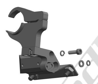
STEP 7 - Reinstall the BODY ASSEMBLY. Be sure to include the lock washer with the top socket head screw and the lock and flat washer with the bottom socket head screw as shown above. NOTE: there are extra lock and flat washers included in the tool kit just in case you happen to misplace one.
