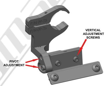
STEP 8 - Install your radar detector onto the mount. Use the adjustments shown above to adjust the RD to your desired position. We recommend adjusting the RD as close to the bottom of your mirror as you can. Be sure to tighten all adjustment screws after the adjustments are made.
