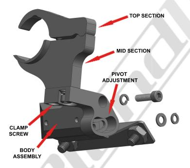
**STEP 3** - The BODY ASSEMBLY must be removed to gain access to the CLAMP SCREW. Remove the two socket head screws as shown above. Be sure to remove the lock washer with the top screw along with the lock washer and flat washer with the bottom screw.
